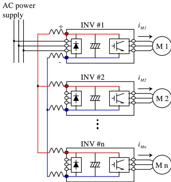
➤ **Pay attention to the selection of the main inverter (#1) because all the input current flows through the rectifier bridge of this inverter. (\*2)**
