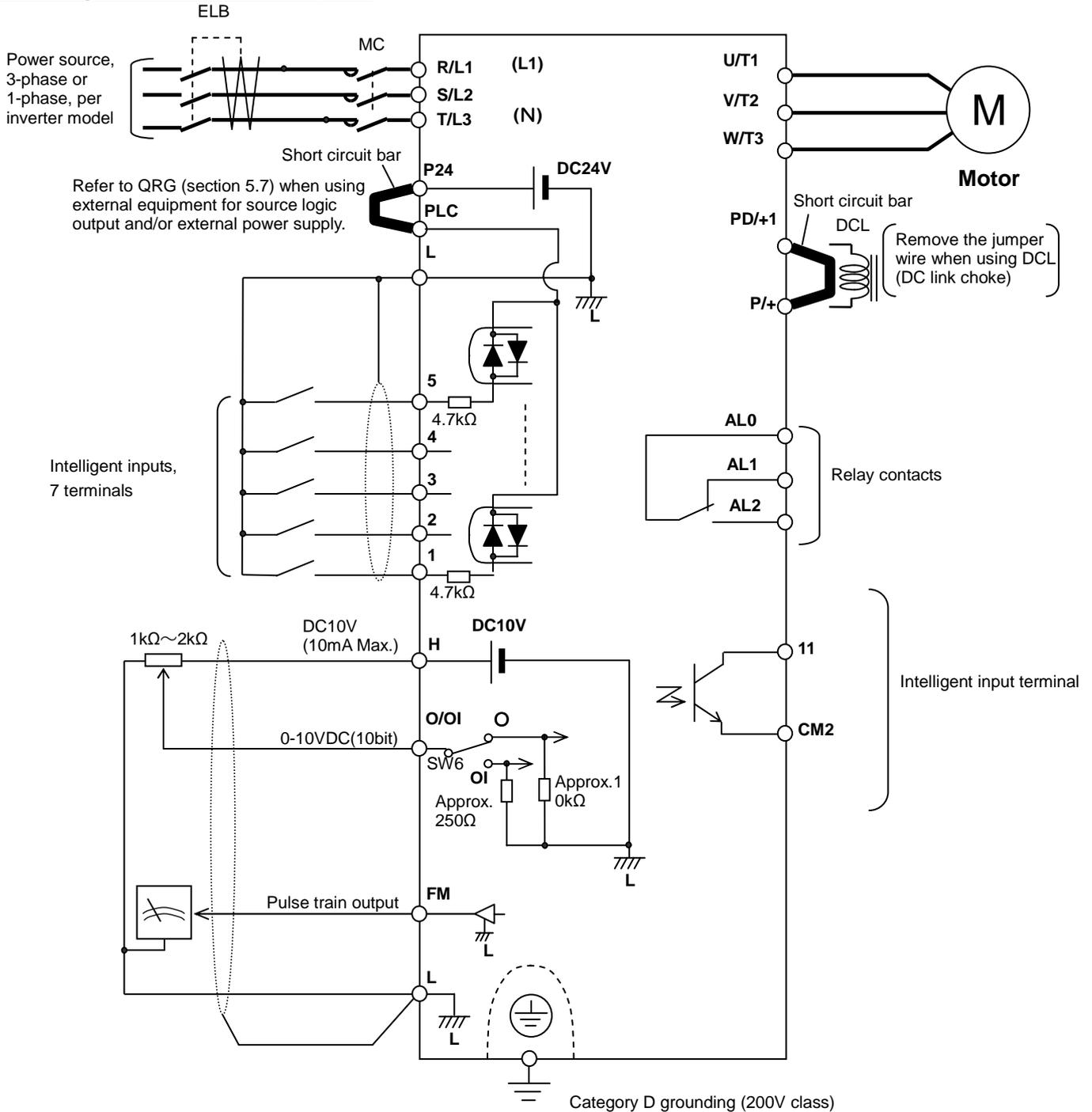
Note 1) Above shows an example of voltage (O) input. Changeover of SW6 must be done in case of current (OI) input. (Refer to page 9).
