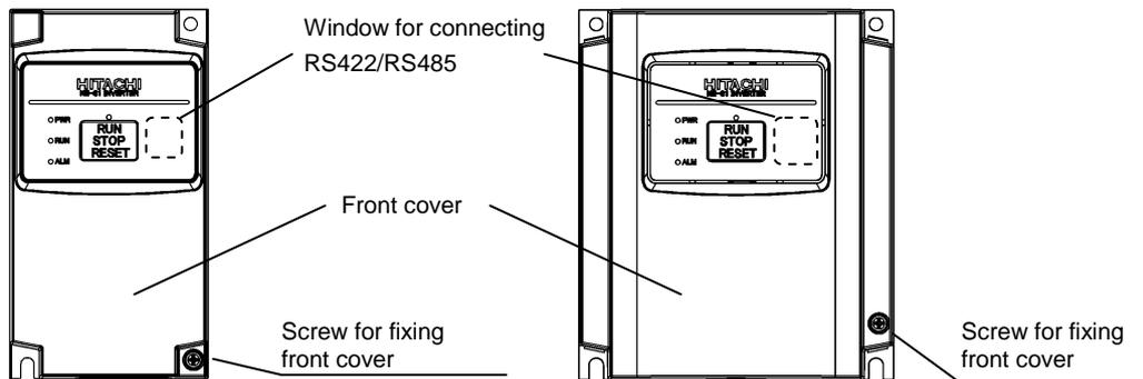
(2) It is necessary to make window on the front cover when using remote operator (OPE-S/SR/SBK/SRmini, WOP), Modbus-RTU, or PC software (ProDriveNext). See above for the position of the window.
