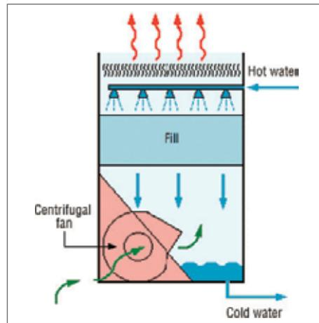
Typical Evaporation Open Tower with Counter Flow
